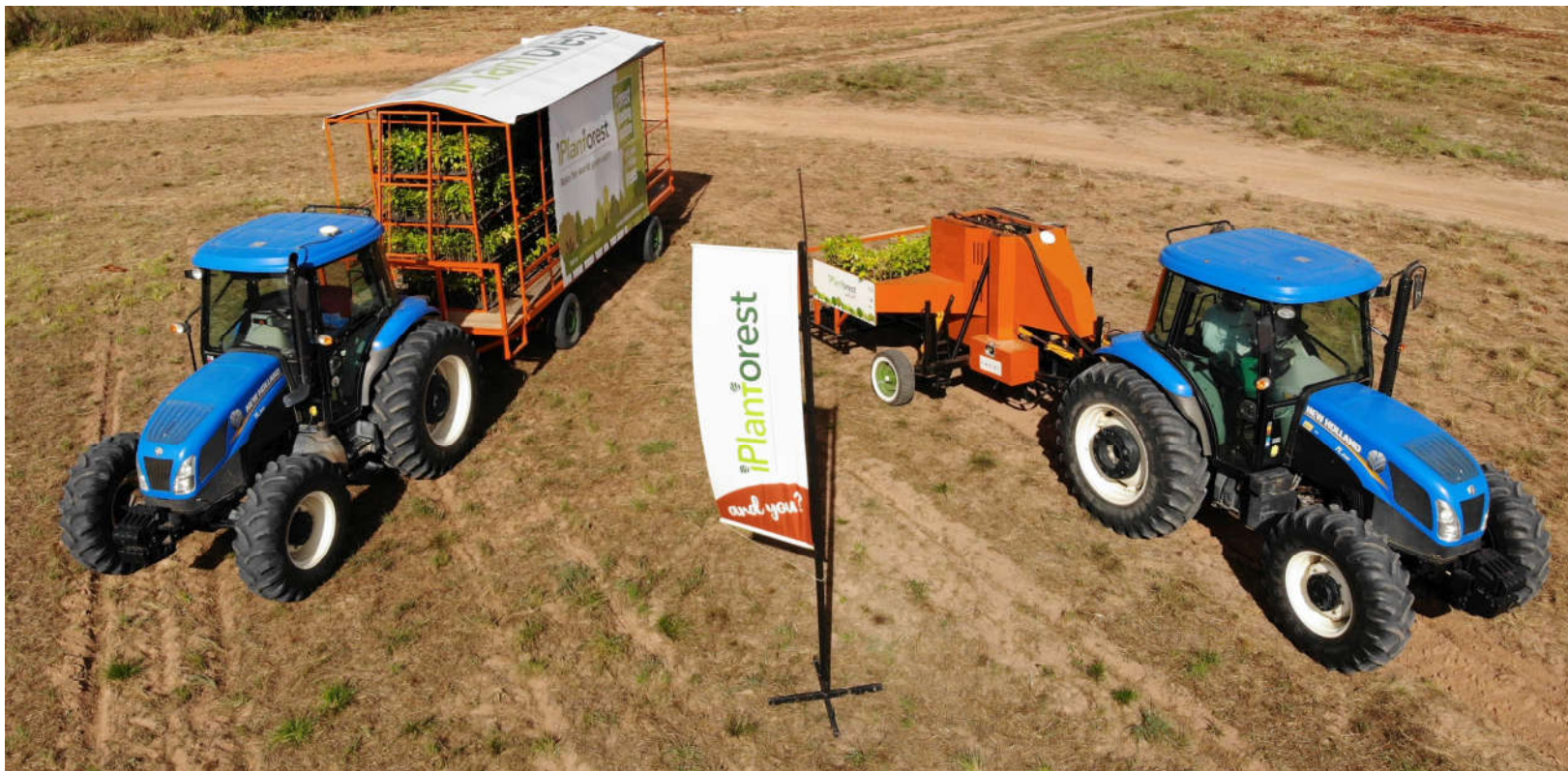
Seedling transport cart and planting machine
